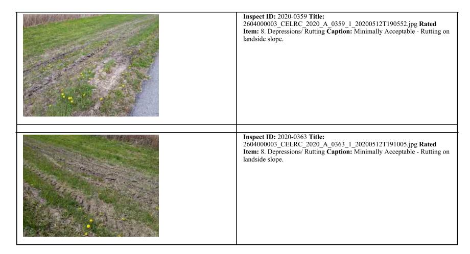
**Photos**For use during Initial and Continuing Eligibility Inspections of levee segments / systems
