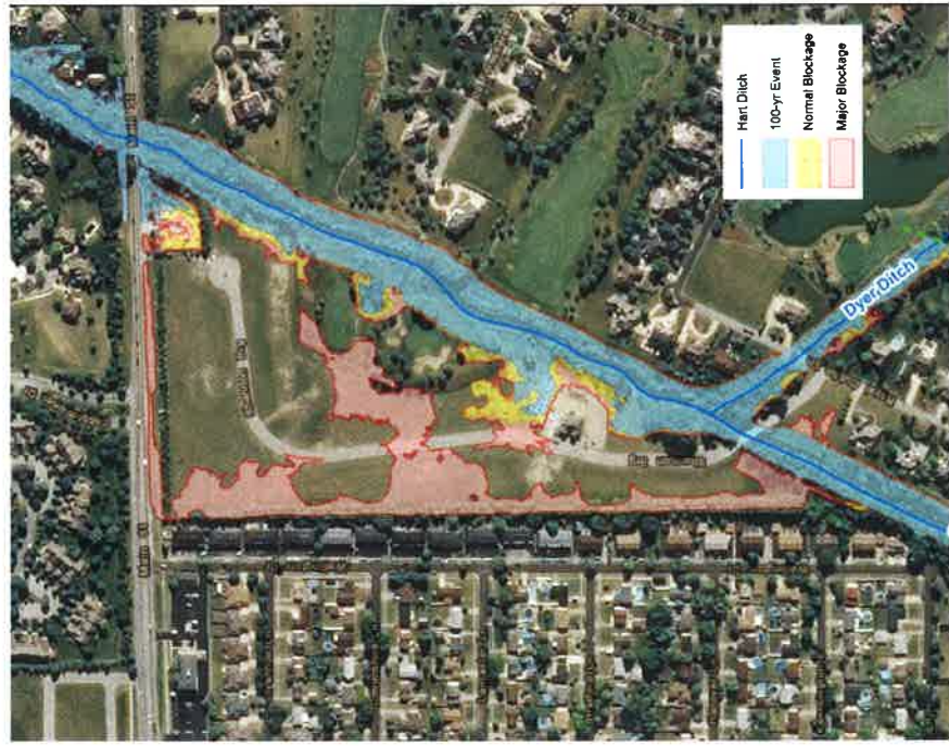
Potential flooding area due to blockage
